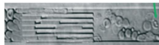
Figure 2. Microfluidic canal constricting RBC resulting in schistocyte-like formation identified with green arrow.
