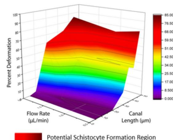
Figure 5. 3D graph of percent plastic deformation of erythrocytes (z-axis and color spectrum) as a function of canal lengths in μm (x-axis) and flow rate in μL/min (y-axis). Flowrate is directly related to shear rate (s<sup>-1</sup>).
