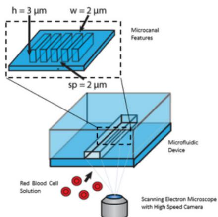
Figure 3. Model of experimental microfluidic system. Each device is comprised of five columns that form "microcanals" that are 2 μm wide and 3 μm tall with lengths varying between 5 μm and 45 μm.
